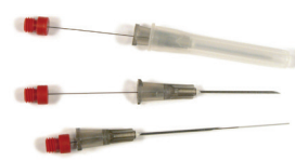
Figure 4. Tip and Probe Biocompatible SPME Configurations
