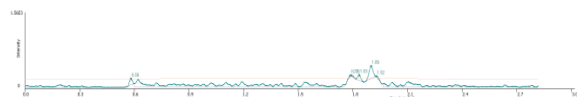
Figure 3: EIC for 0.005ng/mL ME pre spiked plasma following SPE cleanup showing the LC-MRM Transition (180.0/148.0)
